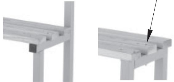
Position the Coat Hanging rail "G" and insert and finger tighten the 4 bolts provided ("H") and ("I").
